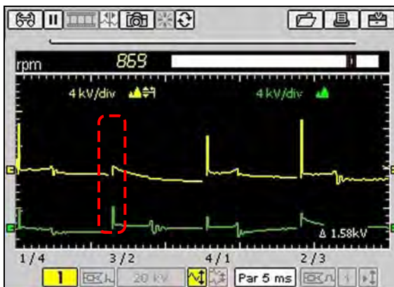
Figure D-8 Sample shorted spark-plug detected
