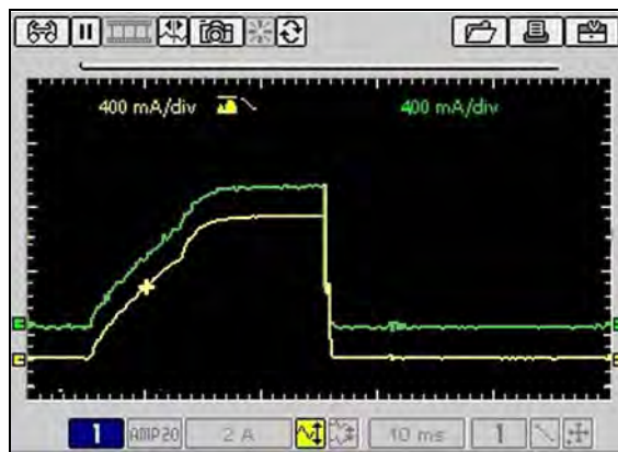
Figure C-7 Sample Noise Filter—two low amp scope probes
